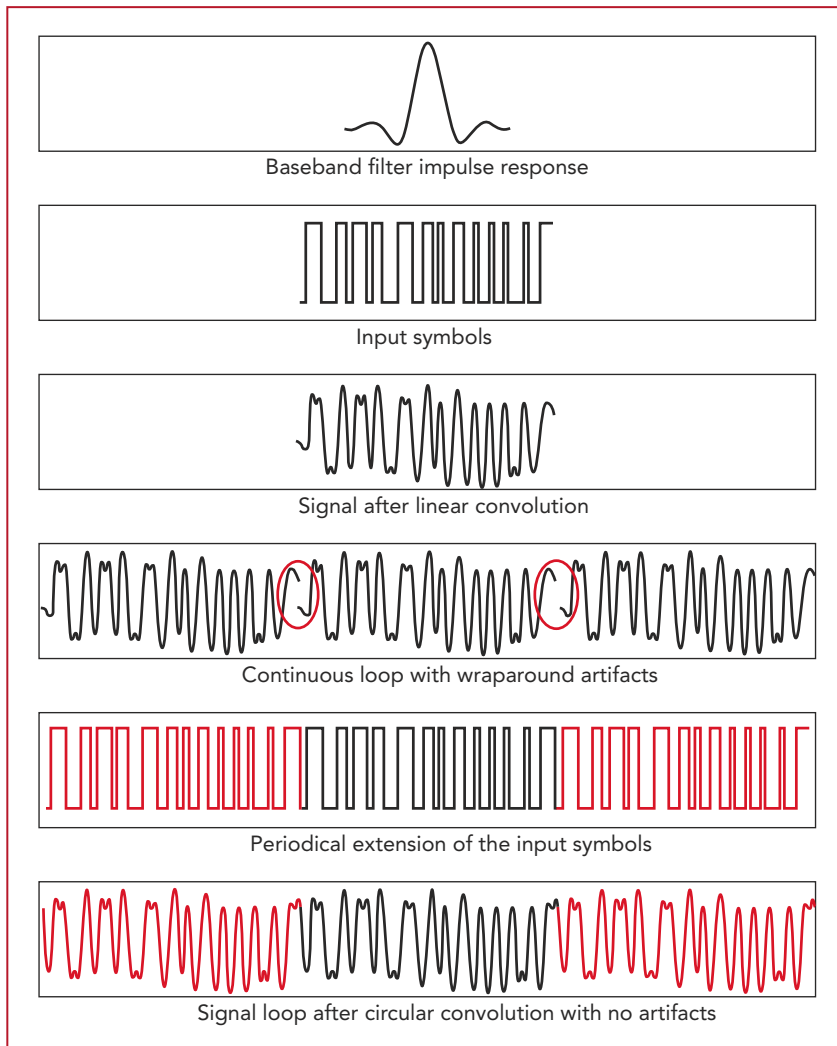
FIGURE 3. Circular convolution is the key to obtaining self-consistent signals that can be looped seamlessly.
